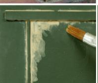
Use a flat brush moist with White Spirit and blend in the paint proximally 10 minutes after it is applied.
