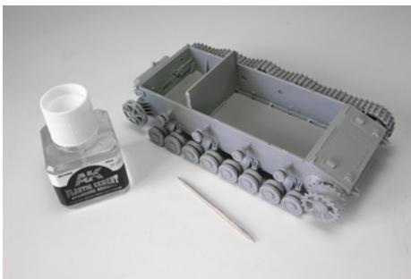
We can use the standard type glue to join large pieces whose joints are not visible after assembly, such as hulls or turrets of vehicles, fuselage halves of aircraft or the ship hulls.
