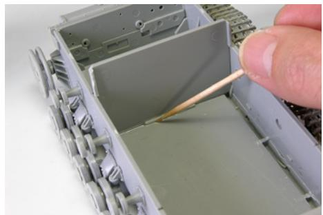
After applying the adhesive along the joint, we can use a wooden toothpick to distribute it into the recesses and less accessible areas. Once it fully cures, the resulting joints are super resistant and the pieces cannot be separated from each other since the plastic in the contact area has completely melted.
