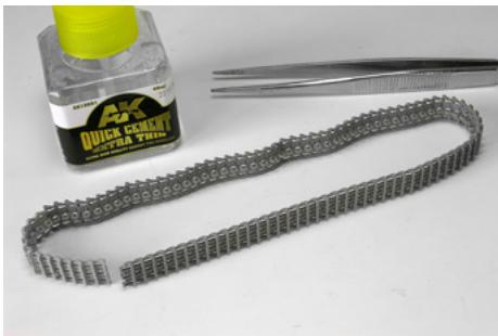
We must place and join each link until completing the track run, sealing the joints with the quick adhesive. In result, we will be able to manipulate the track run for a few minutes as it will remain united and flexible at the same time.
